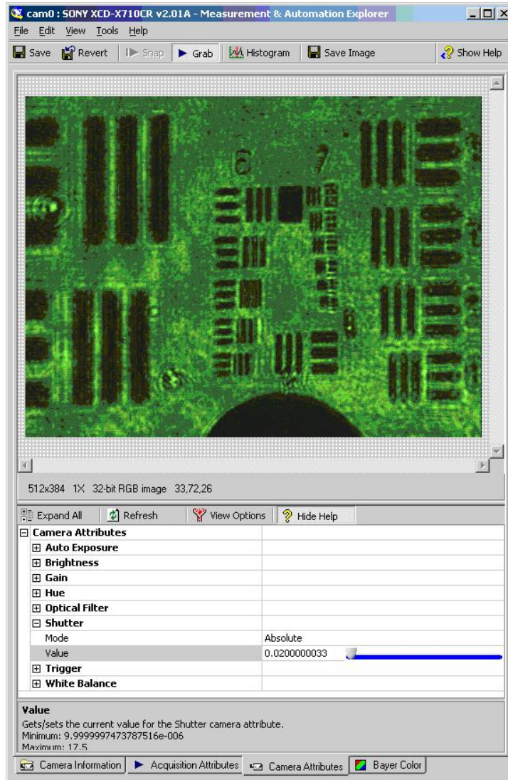
Figure 4.4 TIR camera MAX image of RT chip in glycerin on truncated SFL11 TIR prism; Groups 6 and 7. Tilt compression in phase image is in x-direction. Illumination is with green laser object beam. Shutter speed at 0.02s. Note bubble curvature at bottom FOV; black for loss of signal (LOS).
