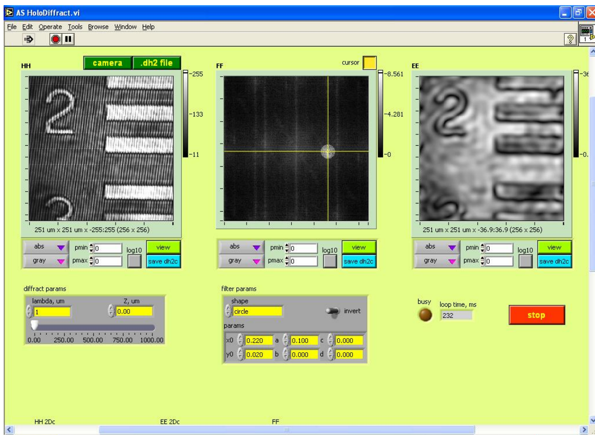
Figure 4.2 AS HoloDiffract Operator's screen; Exp-1A with Michelson unit.
